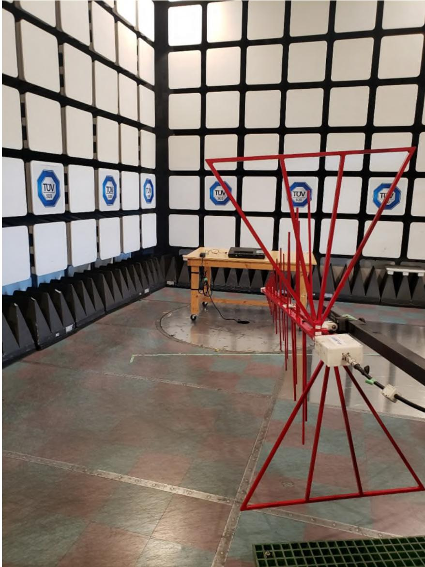
Figure 7 – Radiated Emissions Setup – Photo 1
