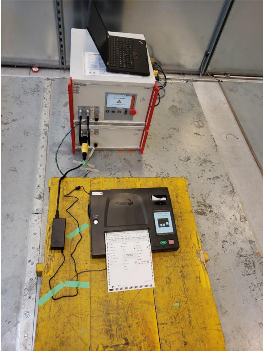
Figure 10 – Electrical Fast Transient / Lightning Surge
