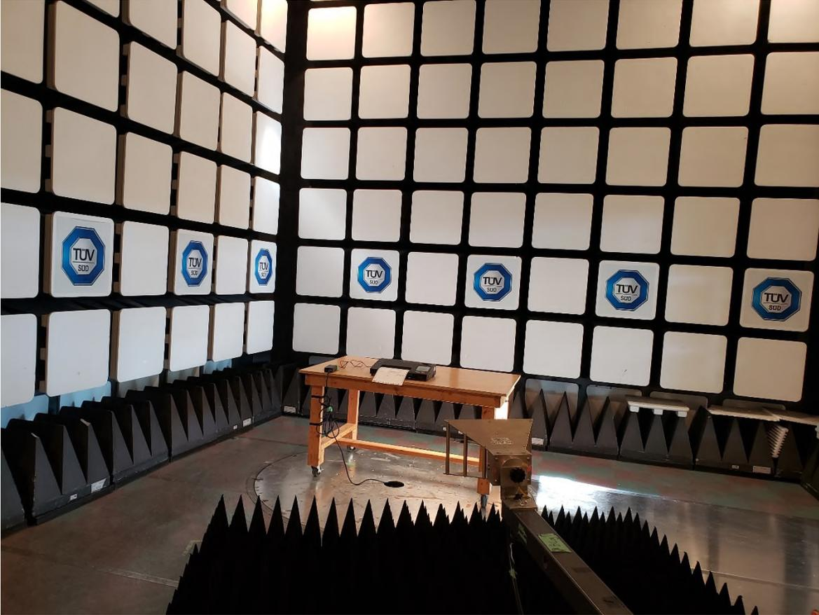
Figure 8 – Radiated Emissions Setup – Photo 2
