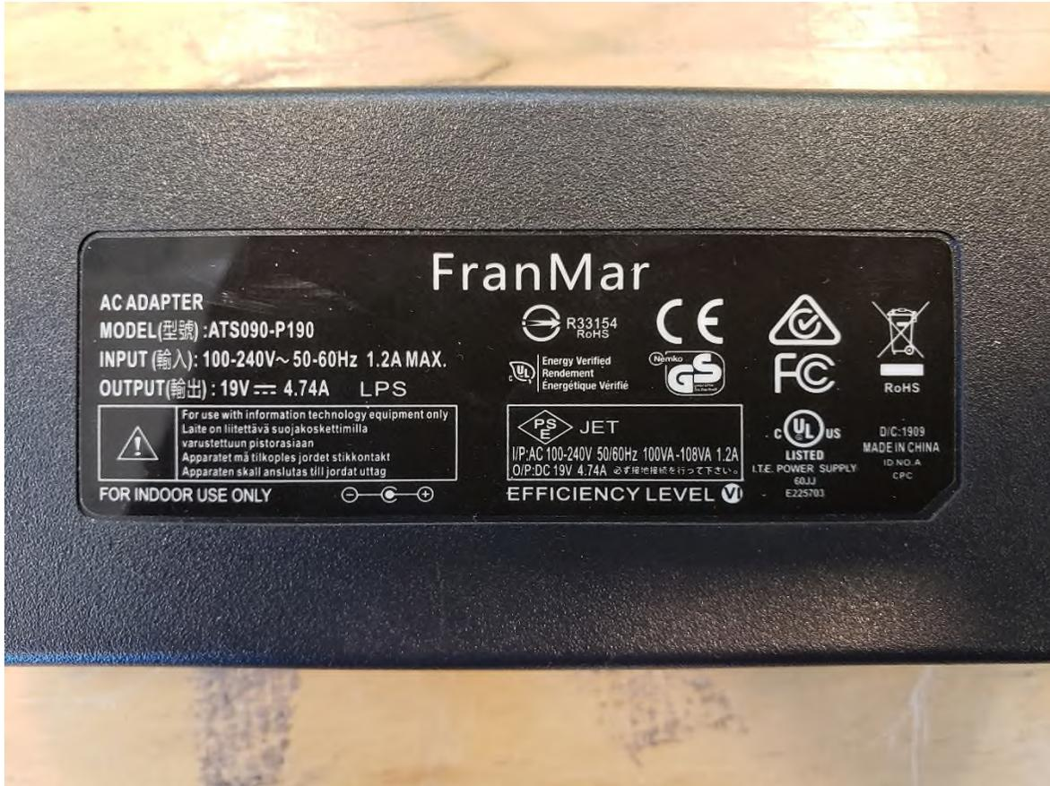
Figure 4 – EUT Power Supply
