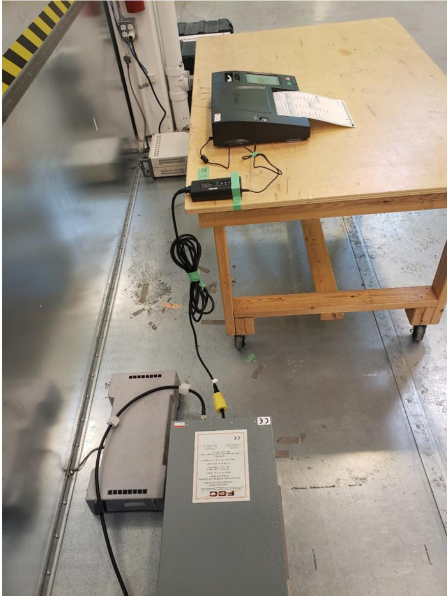
Figure 6 – Power Line Conducted Emissions Setup – Photo 2
