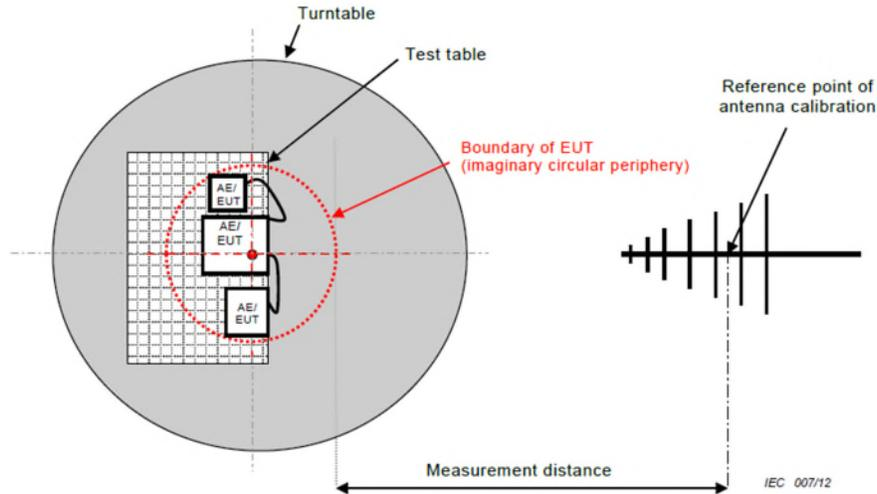
Note: In accordance with FCC Part 15, section 15.31(f)(1), testing was performed at a 3 meter test distance and an extrapolation factor, if applicable, of 20 dB/decade was applied. For example, an extrapolation of 10m to 3m is  $20\log(10/3) = 10.5$  dB.
