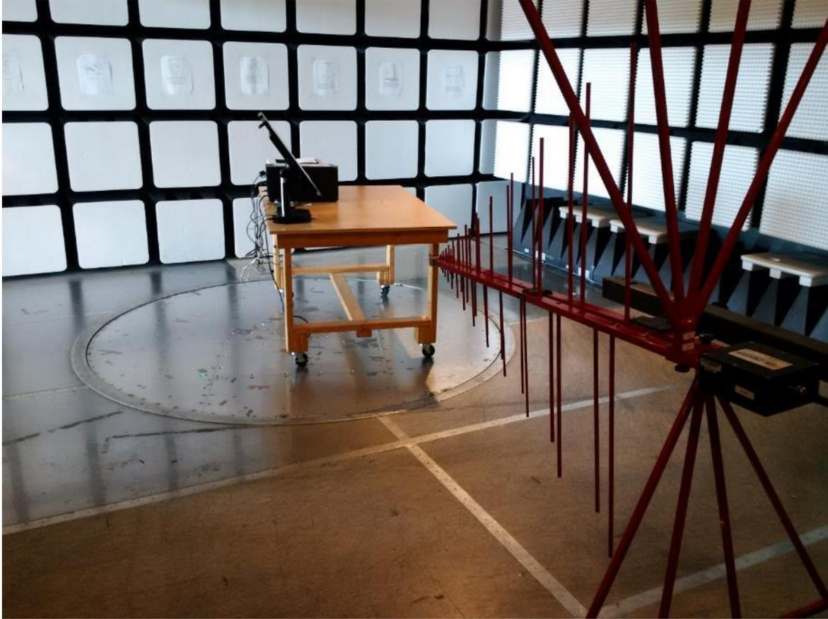
Figure 29 – Radiated Emissions Setup – AVALUE 21" / ICX 21" – Photo 2
