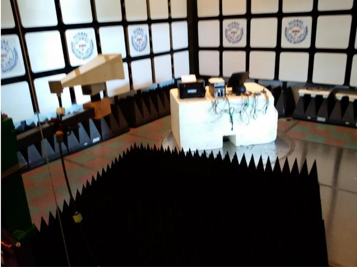
Figure 32 – Radiated Emissions Setup – AVALUE SAMSUNG / SAMSUNG – Photo 2
