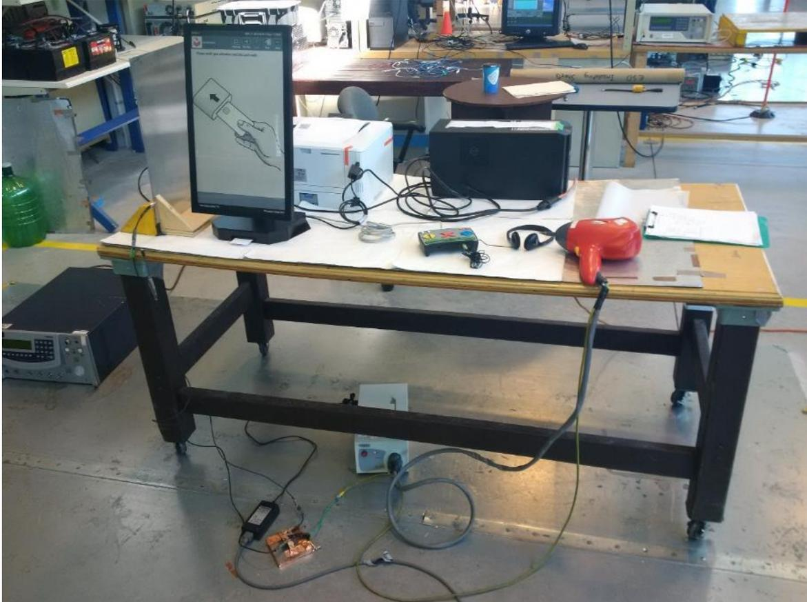
Figure 36 - Electrostatic Disruption Setup – AVALUE 21" / ICX 21"
