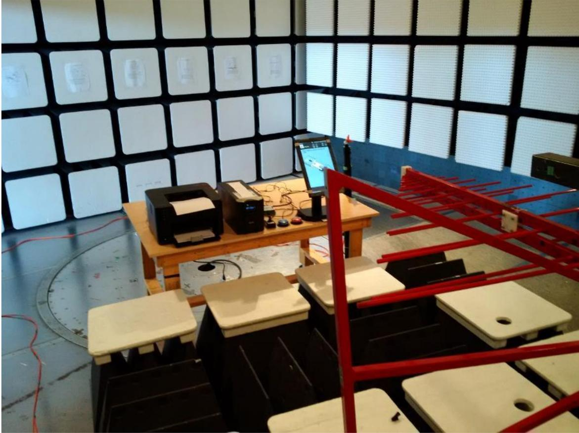
Figure 39 - Electromagnetic Susceptibility Setup – AVALUE 15" / ICX 15"
