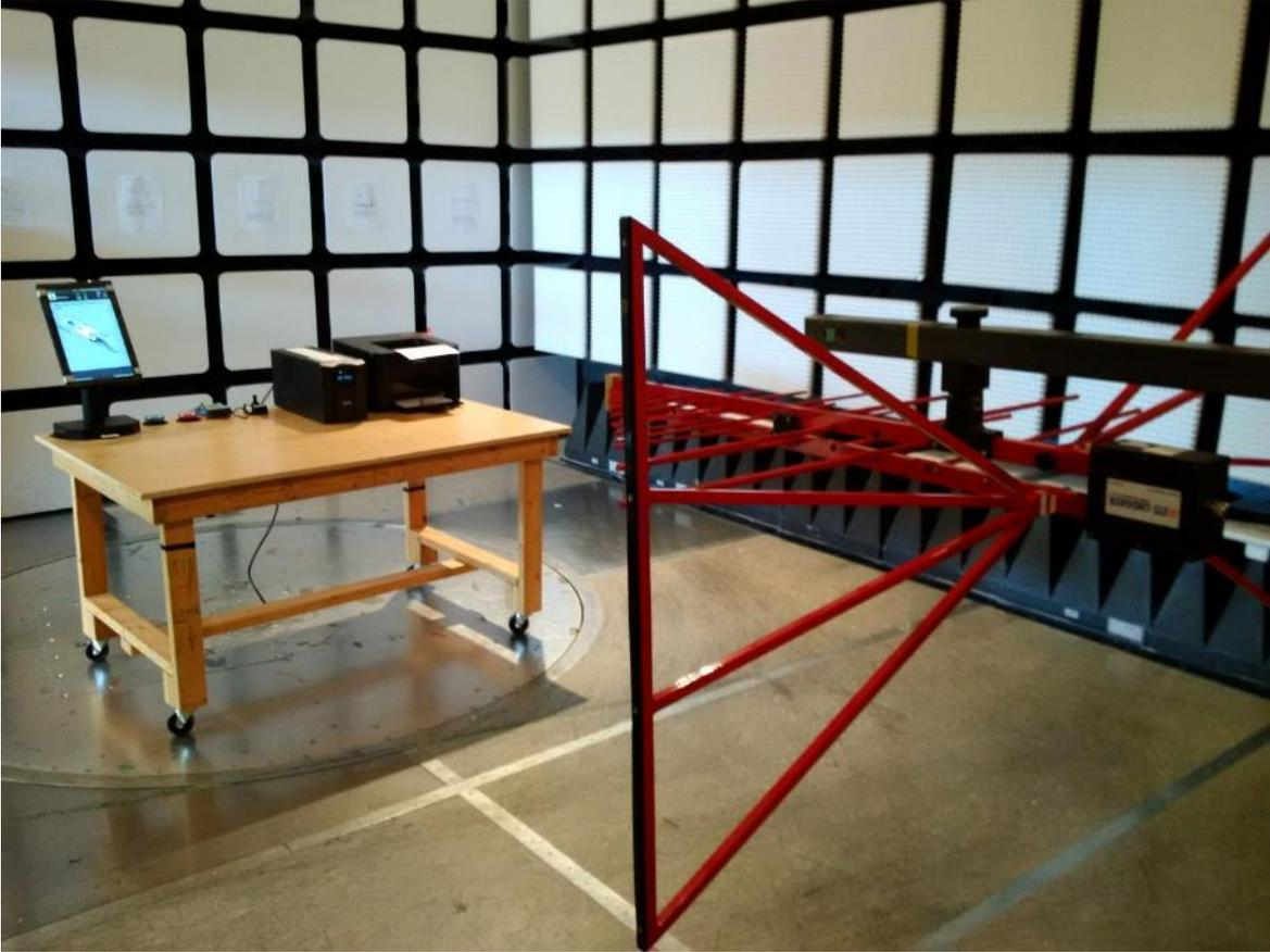
Figure 26 – Radiated Emissions Setup – AVALUE 15" / ICX 15" – Photo 1
