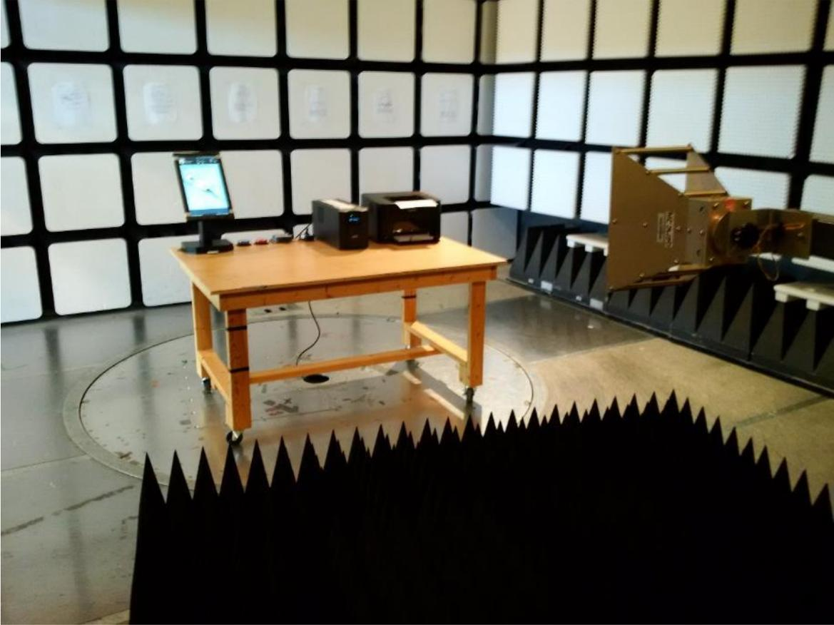
Figure 27 – Radiated Emissions Setup – AVALUE 15" / ICX 15" – Photo 2
