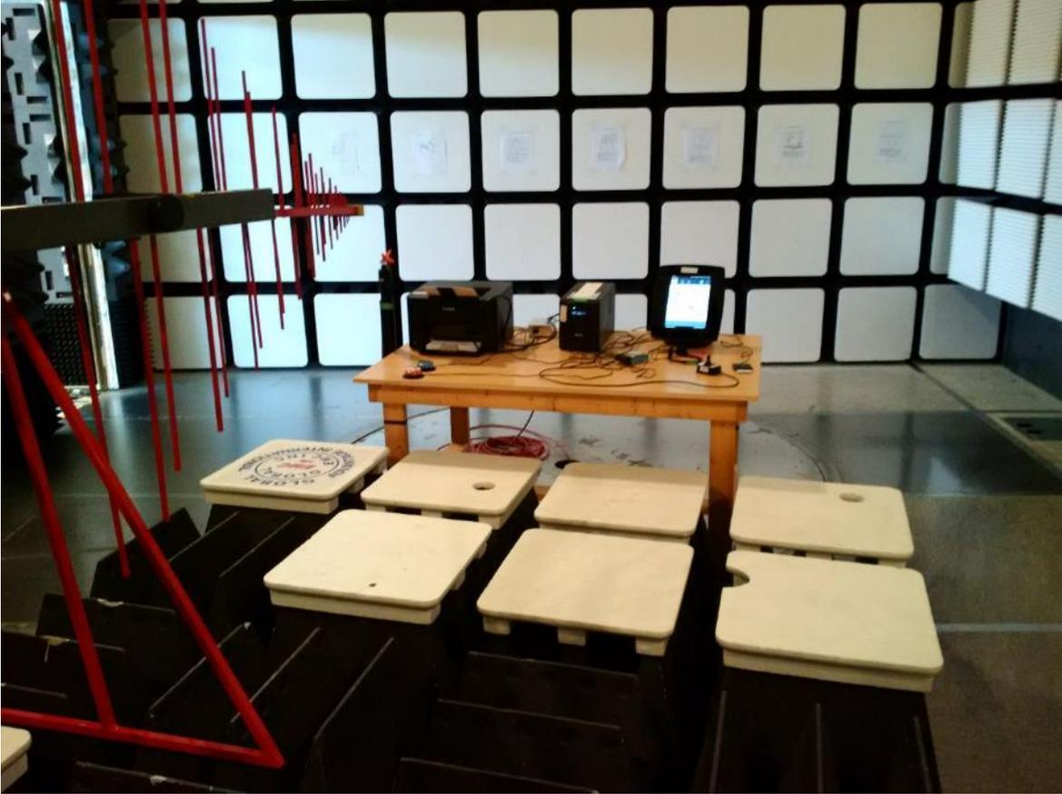
Figure 41 - Electromagnetic Susceptibility Setup
