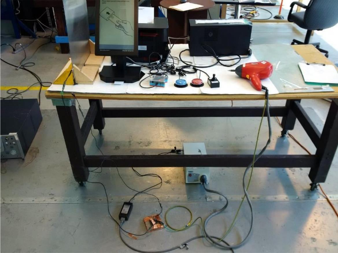
Figure 35 - Electrostatic Disruption Setup – AVALUE 15" / ICX 15"
