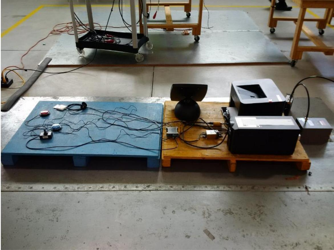
Figure 50 - Conducted RF Immunity – AVALUE SAMSUNG / ICX SAMSUNG
