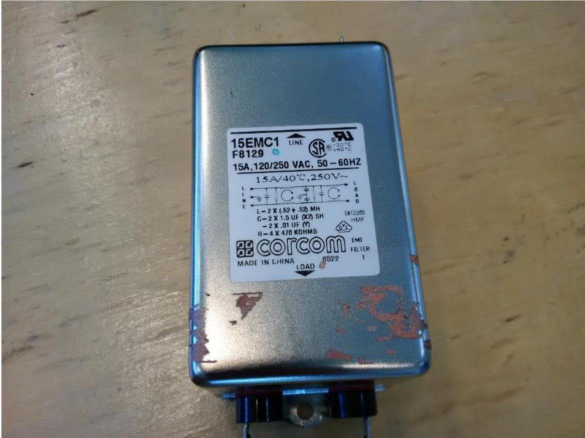
Figure 16 – EUT Close Up – CORCOM Filter
