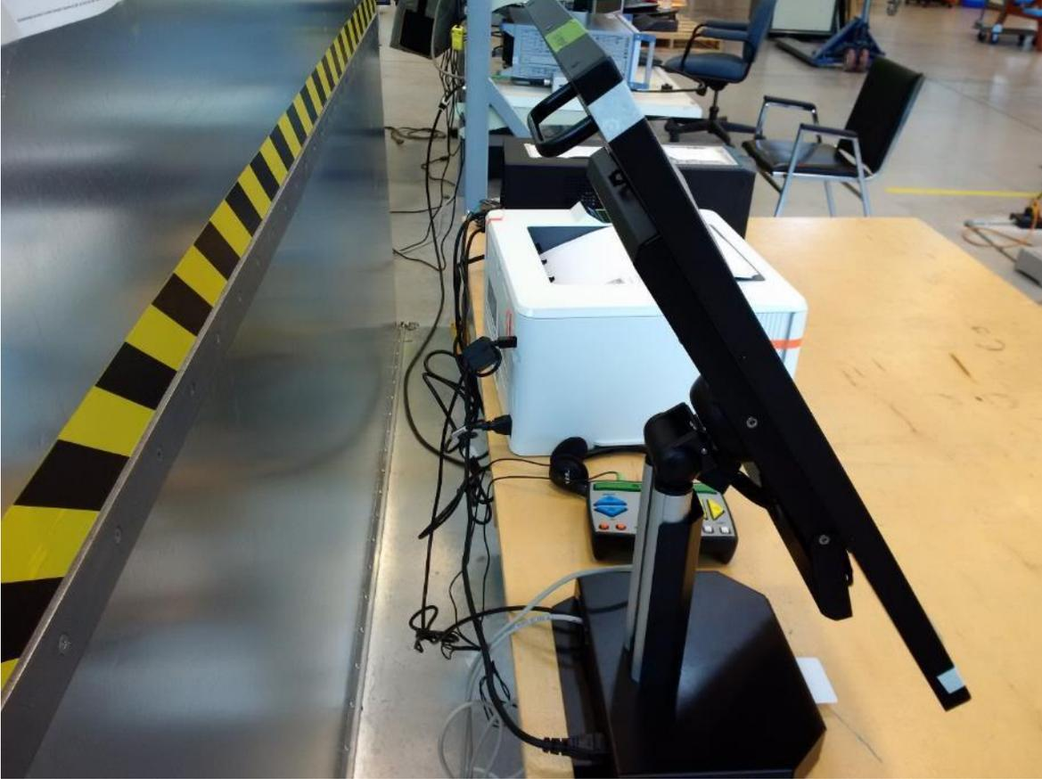
Figure 20 – Conducted Emissions Setup – AVALUE 21" / ICX 21" – Photo 2
