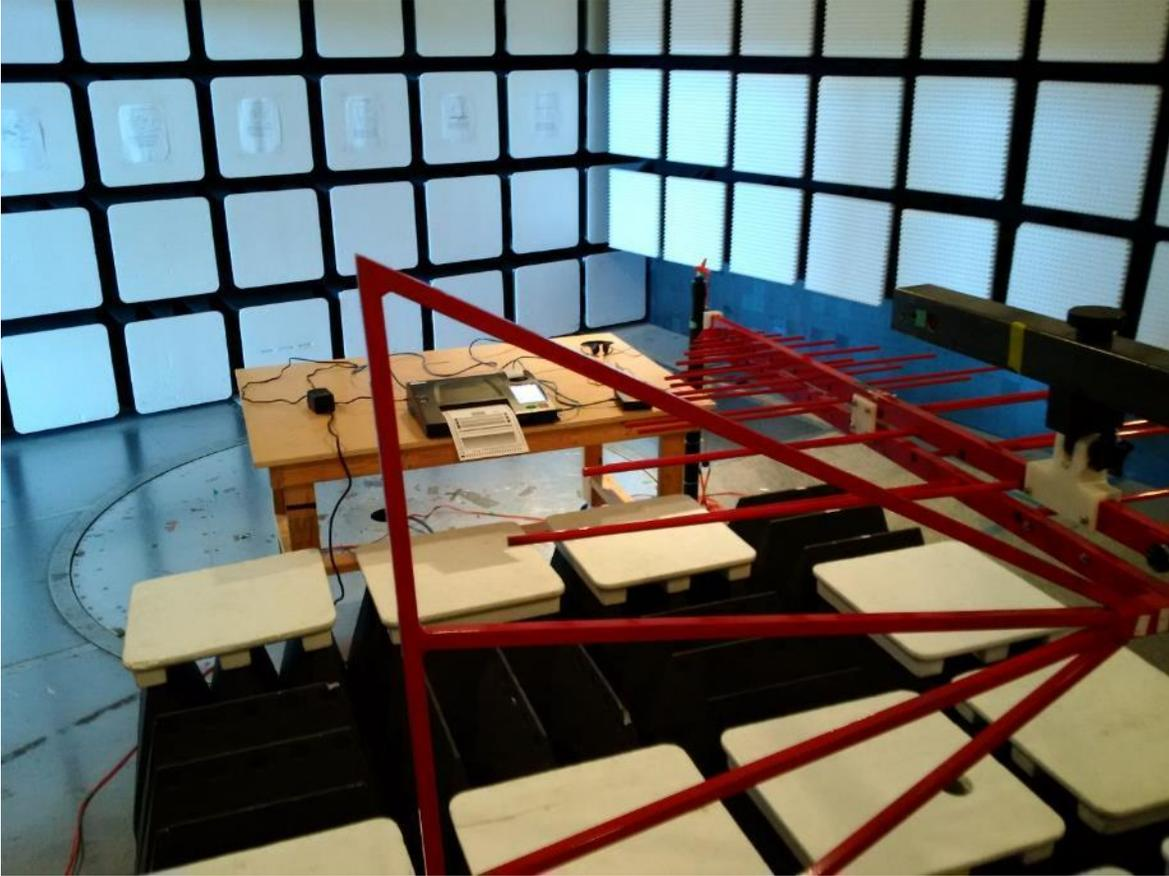
Figure 42 - Electromagnetic Susceptibility Setup – PCOS 320C / ICP
