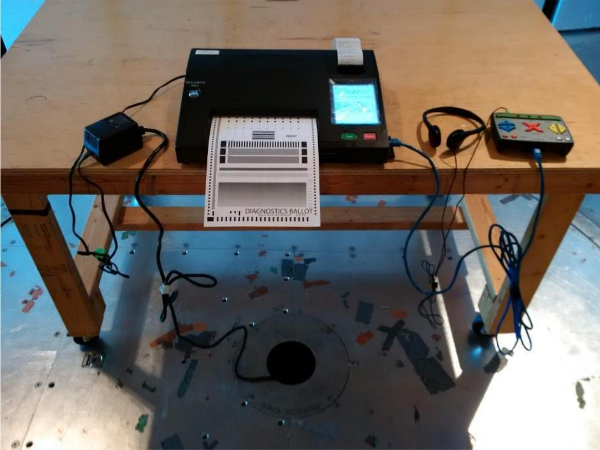
Figure 33 – Radiated Emissions Setup – PCOS 320C / ICP – Photo 1
