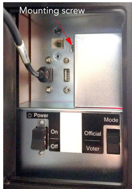
4. Install a wire seal via the available attachment hole on the right side of the box, securing the box to the access compartment.
