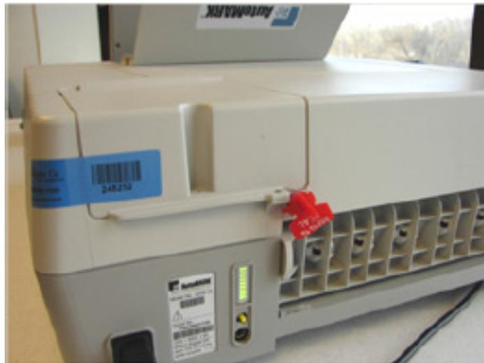
Additional seals can be used on the AutoMARK to prevent unauthorized access to the SBC casing and USB port. Only an ES&S-certified technician or trained vendor technician should apply these seals.
