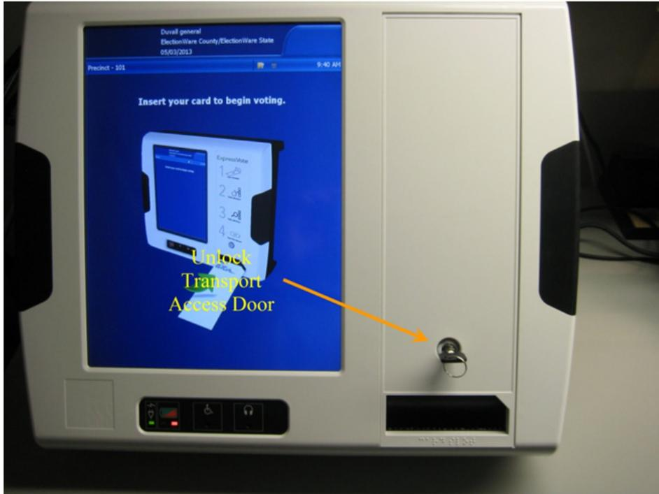
2. Open the transport access door. The prop rod supports the door in the open position.
