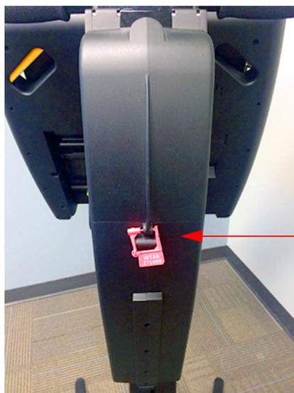
A seal here secures the container door. Leave in place during voting.
