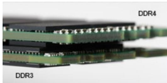
**Figure 2. Thickness difference**
