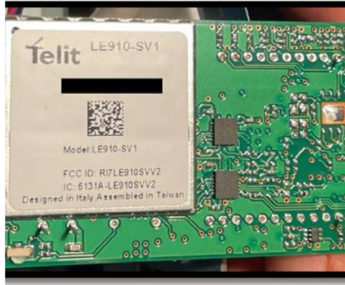
Telit System 4G Wireless Modem Installed on ES&S DS200 Motherboard
