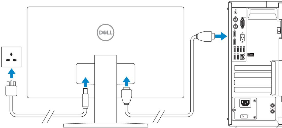
**NOTE:** If you ordered your computer with a discrete graphics card, the HDMI and the display ports on the back panel of your computer are covered. Connect the display to the discrete graphics card.
